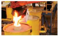
Mercury's exclusive pressurized lost-foam foundry produces more-intricate castings that require fewer fasteners for lighter weight and increased reliability.
