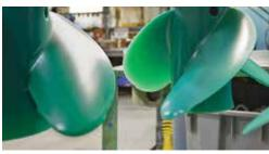
Mercury produces the best performing propellers. All stainless steel props begin as a perfect wax replica of the final product.
