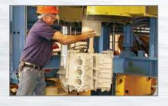
Mercury's exclusive pressurized lost-foam foundry produces components that are stronger, lighter and require fewer fasteners for top-notch reliability, strength, and lower weight.
